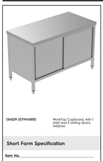
Enhanced stability and solid construction thanks to the welded frame and legs. The 50mm high worktop in 304 AISI stainless steel, with Scotch Brite finishing 15/10 mm in thickness, has antidrip edges and welded corners. 18mm thick undertop waterproof reinforcement, it's completely waterproof, double-sided laminated and 100% recyclable. Sound-deadned double walled sliding doors on roll bearings with end limit stop (7/10 in thickness in 304 AISI stainless steel).
